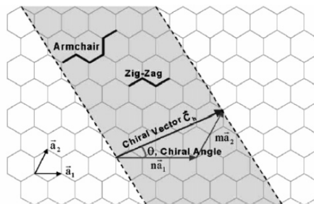
Figure 2. Schematic diagram showing how a hexagonal sheet of graphene is "rolled" to form a carbon nanotube. The rolling shown in the diagram will form a (3,2) nanotube. Reprinted with permission from ref 16. Copyright 2001 Elsevier.
